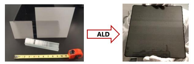
Incom Glass Capillary Arrays (GCAs) are available in sizeable dimensions (left: 33 mm round, 108 mm and 203 mm square) and are functionalized by ALD to yield Microchannel Plates (MCPs) as presented at a 203x203 mm sized example (right).
