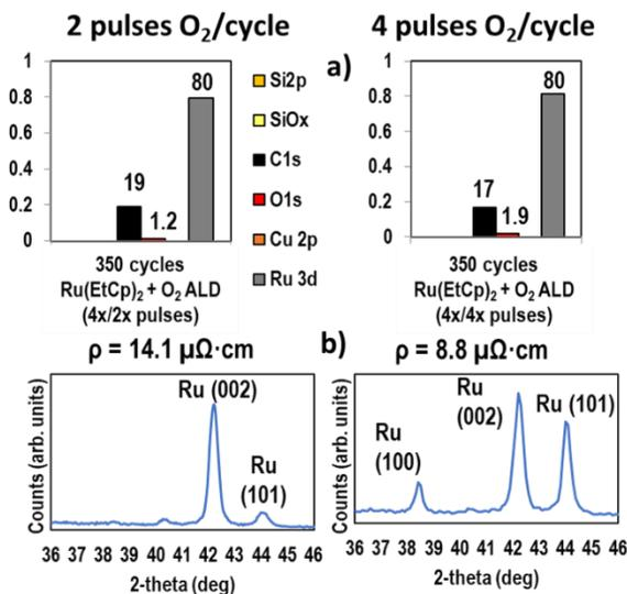
**Fig. 4. Resistivity-oxygen dose relationship for Ru ALD using Ru(EtCp)<sub>2</sub>.** At 2 pulses/cycle, growth rate was 0.9 Å/cycle, while at 4 pulses/cycle, growth rate was 1.0 Å/cycle. a) Oxygen content of both films was sub 2%, with the 2 pulse and 4 pulse/cycle films having a resistivity of 14.1 and 8.8  $\mu\Omega\cdot\text{cm}$ , respectively. b) XRD and XRR of the films shows that the Ru(002) peak is dominant, but the Ru(101) grain size increases from 18.4 nm to 28.0 nm.
