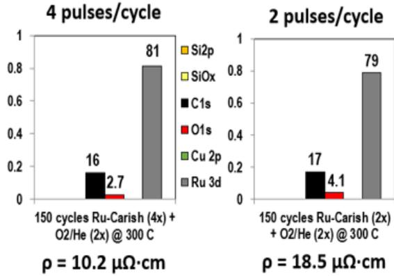
**Fig. 1. Effect of Ru-Carish pulses on Ru resistivity.** At 300 C, after 150 cycles at 2 pulses per cycle of Ru-Carish, the film contains roughly 4.1% O, with a resistivity of 18.5  $\mu\Omega\cdot\text{cm}$ . Doubling the number of pulses reduces the percentage to 2.7%, with a decrease in resistivity to 10.2  $\mu\Omega\cdot\text{cm}$ .
