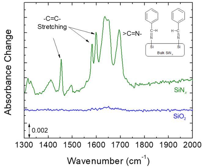
Figure 1: Infrared absorbance change of the infrared active region for a  $\text{SiN}_x$  (green) and  $\text{SiO}_2$  (blue) surface after exposure to benzaldehyde at a substrate temperature of  $70^\circ\text{C}$ .
