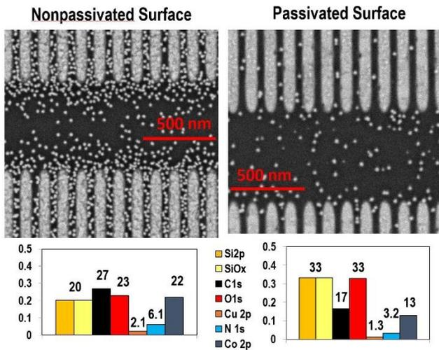
**Fig. 1. 200 Cycles of Co(DAD)<sub>2</sub> + TBA at 180°C on a Patterned Cu/SiO<sub>2</sub> structure.** The Cu stripes are gray and the SiO<sub>2</sub> areas are black. (left) After 200 cycles on the unpassivated sample, unwanted Co nuclei are observed close to the Co/Cu stripes. (right) On a passivated sample, the density of unwanted nuclei is 4x lower and more uniform across SiO<sub>2</sub>.
