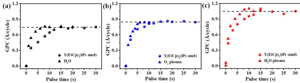
Figure 1 Saturation plots of ALD  $Y_2O_3$  films at a substrate temperature  $200\text{ }^\circ\text{C}$  with  $Y(\text{EtCp})_2(\text{iPr-amd})$  and (a)  $H_2O$ , (b)  $O_2$  plasma and (c)  $H_2O$  plasma as reactant. The data determined by *in-situ* spectroscopic ellipsometry versus ALD cycle number.
