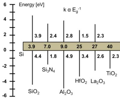
Fig. 1. Band offsets between silicon and different high-k materials. Ultra-thin high-k materials could promote the formation of quantum wells by taking advantage of these offsets. Resonant tunneling could be promoted for these materials.
