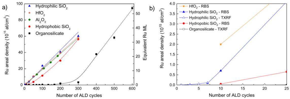
Figure 1: a) Ru coverage measured by Rutherford Backscattering Spectrometry (RBS) for increasing ALD cycle number on -OH terminated hydrophilic SiO<sub>2</sub>, HfO<sub>2</sub>, Al<sub>2</sub>O<sub>3</sub>, Si-O-Si terminated hydrophobic SiO<sub>2</sub>, and Si-CH<sub>3</sub> organosilicate glass, b) inset for low ALD cycle number, showing Ru RBS and Total X-Ray Fluorescence Spectrometry (TXRF) for the initial ALD cycles. Closed lines are provided as a guide to the eye.
