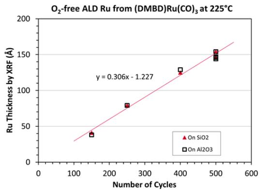
Fig. 1. Linear growth of O<sub>2</sub>-free Ru at 225°C
