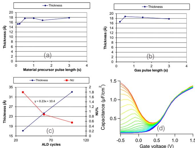
Figure 1. Pulse saturation curves of precursor (a) and (b); and (c) growth rate; and (d) CV characteristic for planar InGaAs MOSCAPs with novel ALD IL
