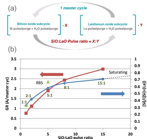
Figure 2. (a) Scheme of lanthanum silicate ALD process; (b) the growth rate and [Si] content of lanthanum silicate process at different pulse ratios
