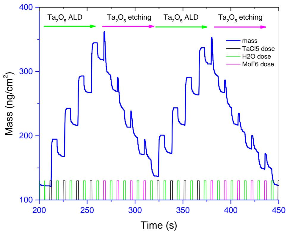
Figure 1: QCM study of  $\text{Ta}_2\text{O}_5$  ALD using  $\text{TaCl}_5$  and  $\text{H}_2\text{O}$ , and  $\text{Ta}_2\text{O}_5$  layer-by layer etching using  $\text{MoF}_6$  and  $\text{H}_2\text{O}$ .
