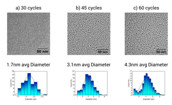
Figure 1 - TEM analysis of PEALD Pt island growth on SiO<sub>2</sub> at a) 30 cycles b) 45 cycles and c) 60 cycles
