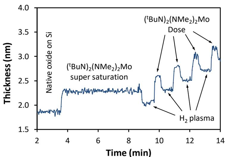
**Figure 1.** Spectroscopic ellipsometry of the first 4 cycles of PE-ALD grown  $\text{MoC}_x$  at  $150\text{ }^\circ\text{C}$  on native silicon dioxide.
