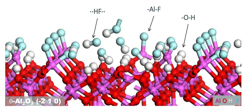
Surface structure computed with DFT for adsorption of multiple HF molecules onto alumina surface in thermal ALE.
