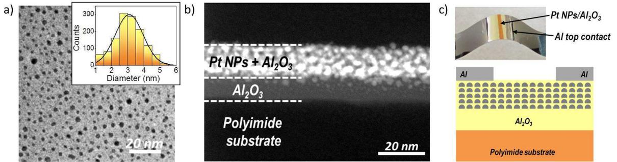
Fig. 1: (a) Bright field TEM image of Pt nanoparticles grown on a 5nm thick Al<sub>2</sub>O<sub>3</sub> film. Inset shows the diameter distribution plot of the Pt NPs. (b) High angle annular dark field – STEM cross section image of a Pt NPs-based strain gauge integrated on a flexible polyimide substrate. (c) Photograph and schematic illustration of a complete flexible strain sensor.
