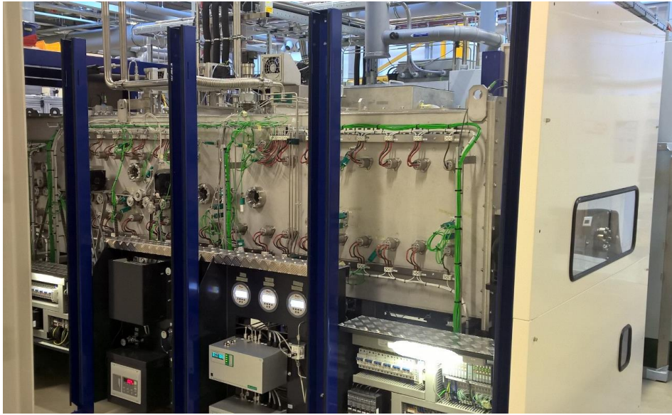
Figure 1. Picture of the sALD section of the large-area sheet-to-sheet spatial atmospheric ALD tool.
