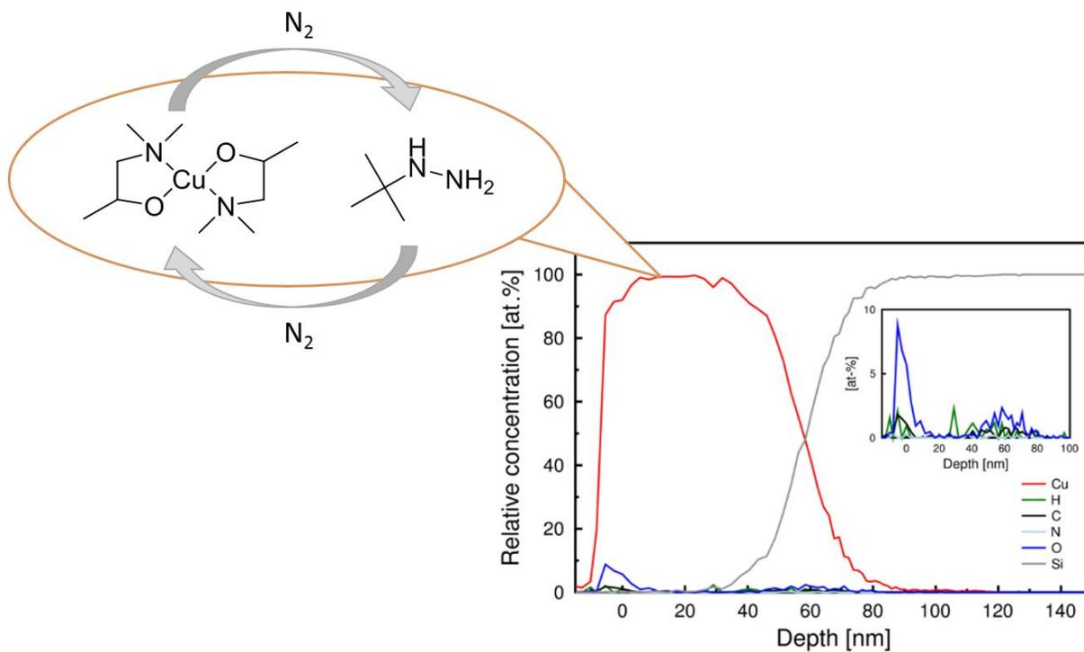
**Figure 1.** ToF-ERDA results of ALD Cu deposited from  $\text{Cu}(\text{dmap})_2$  and TBH at 120 °C.
